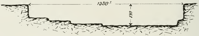
FIG. 18.—Section of King Bros.' large quarry at Thetford.
